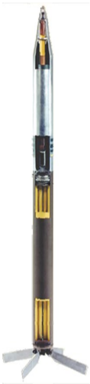
Cut-out of Rocket to be Treated at BGCAPP
